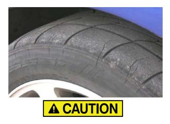
The rubber compounds used in these tires have unique properties that, when compared to other tires, can cause them to lose some of their flexibility when used or handled in conditions below 15°F (-9°C). This loss in flexibility can lead to potential cracking and other damage to the tire.
